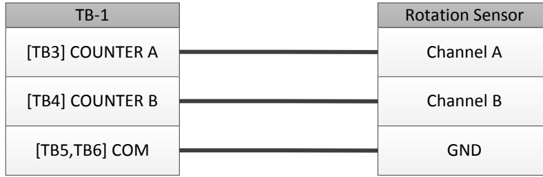
Figure 8 - Connecting rotation sensor with quadrature outputs
