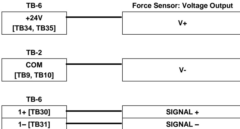
Figure 4.8 – Sensor Hookup – 4 Wire DC Voltage Input
