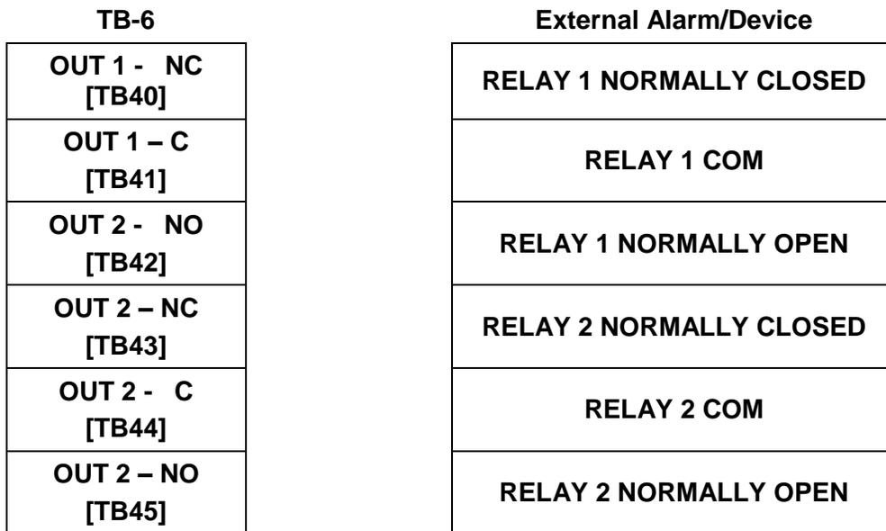
Figure 4.16 – Alarm Output Hookup – 2 Channels
