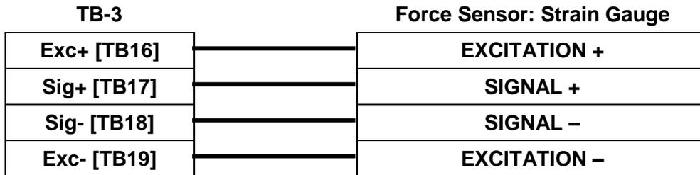
Figure 4.9 - Strain Gauge Input - 4-wire Strain Gauge
