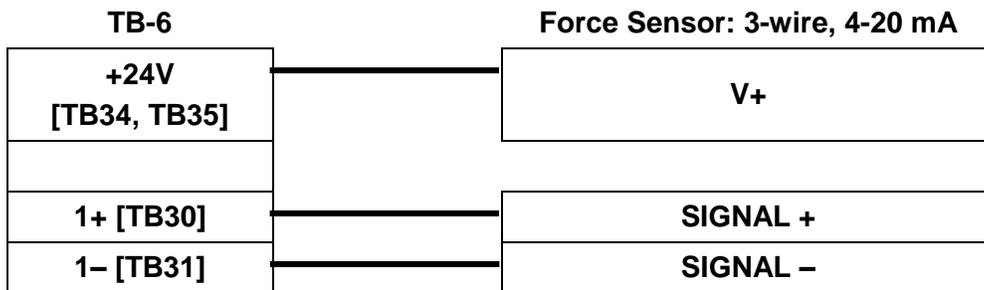
**Figure 4.5 – Sensor Hookup – 3-wire 4-20 mA Signal**
