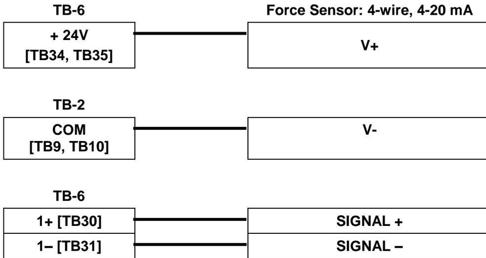
Figure 4.6 – Sensor Hookup – 4 Wire 4-20 mA Signal
