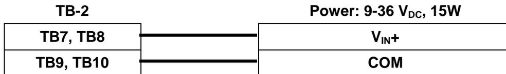
**Figure 4.3 – Local Display Power Hookup – DC Power**
