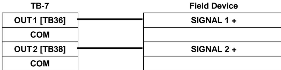
Figure 4.19 – Analog Output Connections – 2 Channels
