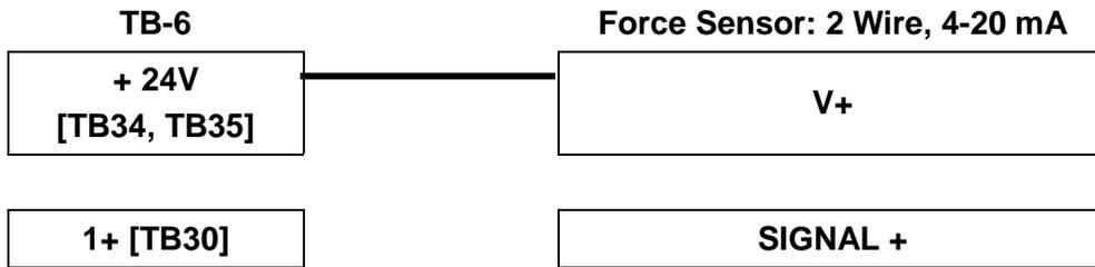
Figure 4.7 – Sensor Hookup – 2 Wire 4-20 mA Signal
