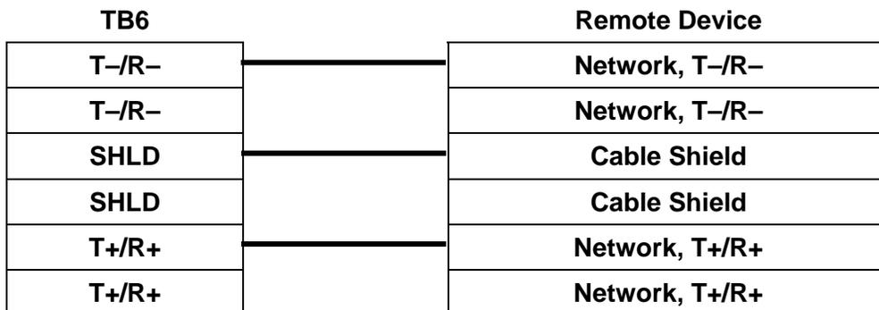
Note: the duplicate terminal blocks are used for daisy chaining multiple units.
