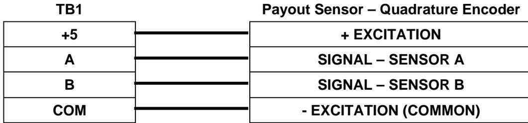
Figure 2.2 – Payout Sensor Hookup – 5VDC Quadrature Encoder
