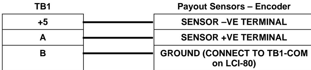
Figure 4.5 - Payout Sensor Hookup - Magnetic Pickup
