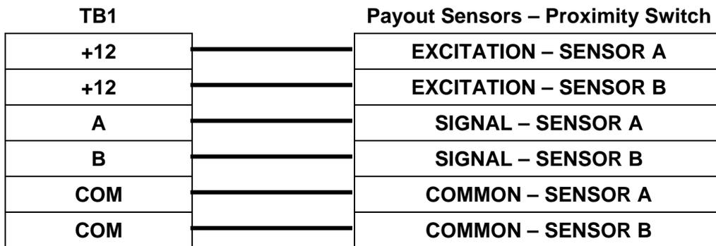
Figure 4.3 - Payout Sensor Hookup - 12V NPN/PNP switches
