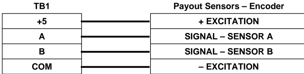
Figure 4.4 - Payout Sensor Hookup - TTL Encoder
