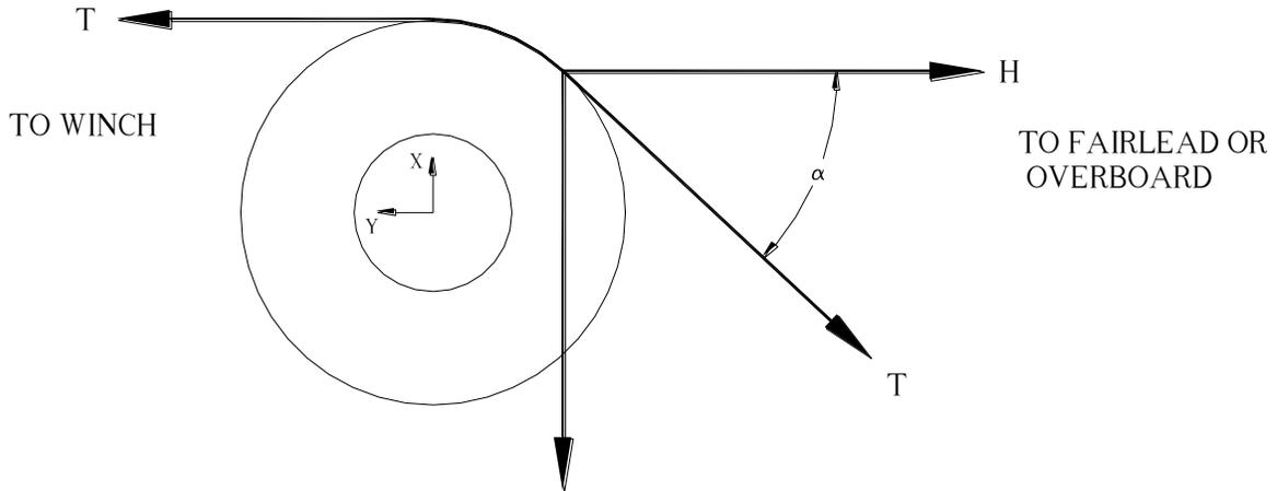
This is the idealized condition where the Y-axis is parallel to the line going to the winch. This is a fixed relationship, but as the equations below show,  $\alpha$  can vary without changing the calculated Tension.
