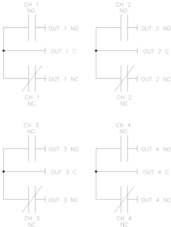
Figure 21 - Digital Output Circuit Schematic
