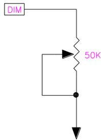
**Figure 32 - Display Contrast Circuit Schematic**
