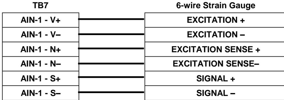
Figure 15 - 6-wire Strain Gauge
