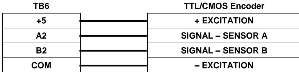
Figure 18 - TTL/CMOS Encoder
