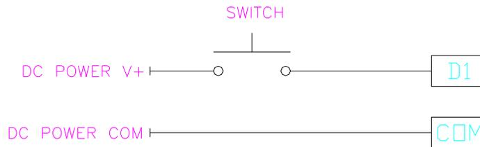
**Figure 23 - Digital Input Using External Voltage Source**
