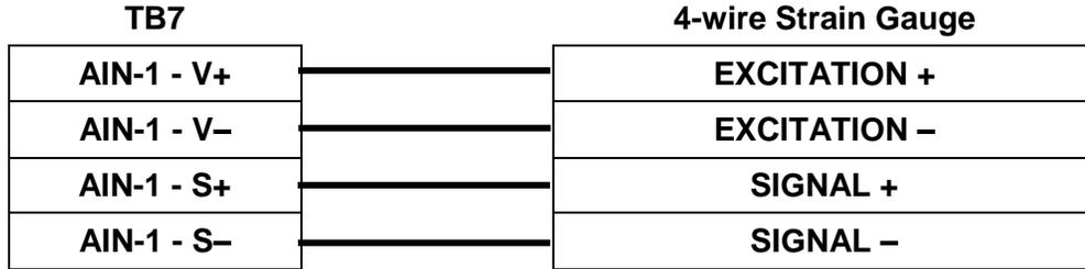
Figure 14 - 4-wire Strain Gauge
