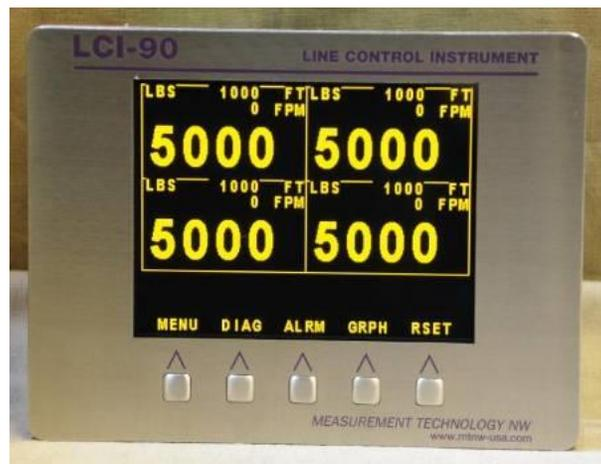
**Figure 47 - Quad Winch Display**
