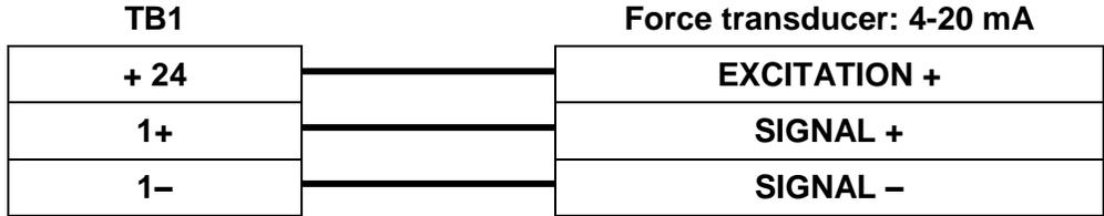
Figure 3 - Force Sensor Connection
