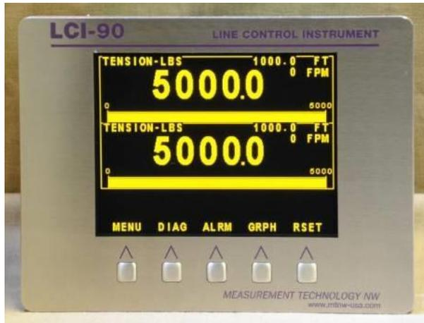
**Figure 45 - Dual Winch Display**
