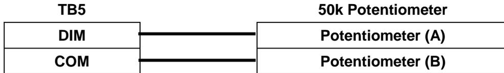
**Figure 33 - Display Contrast Connection**
