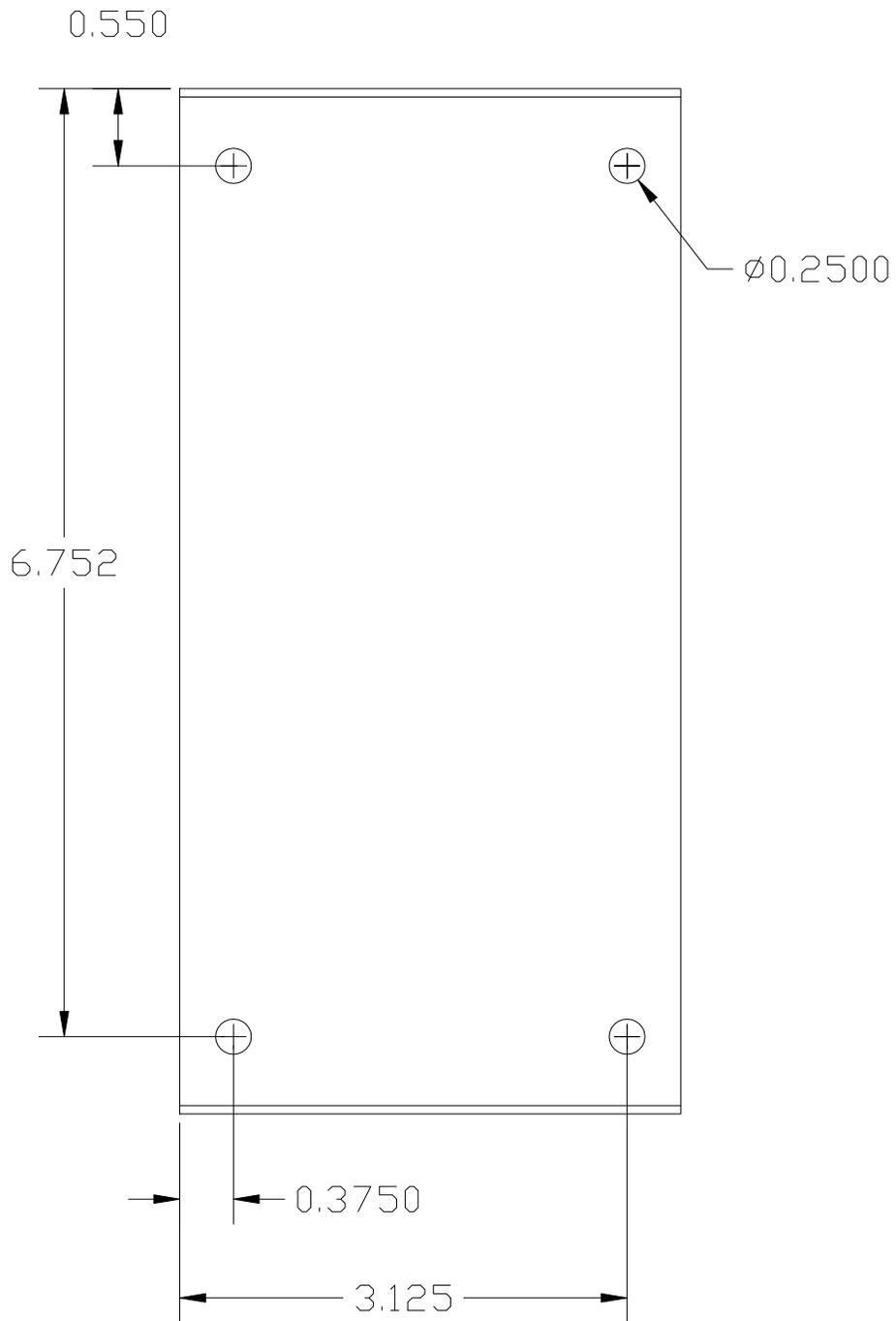
**Figure 71 - LCI-90i Mounting Bracket Footprint**
