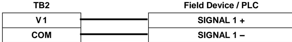
**Figure 25 - Voltage Outputs**
