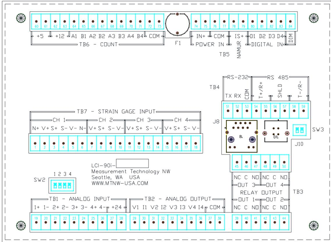
**Figure 70 - LCI-90i Terminal Board Interface**
