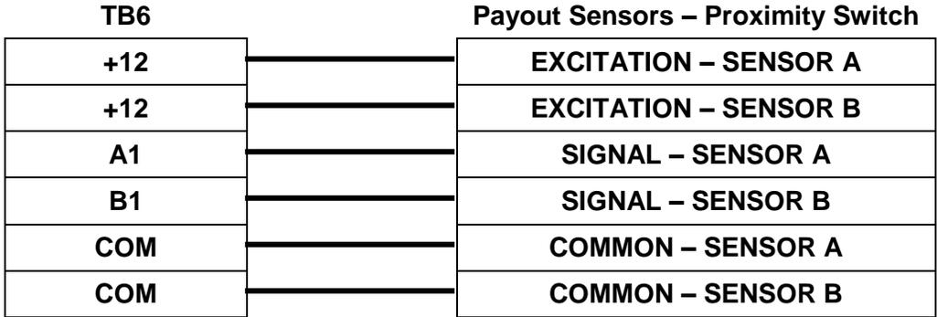
Figure 4 - Count Sensor Connection
