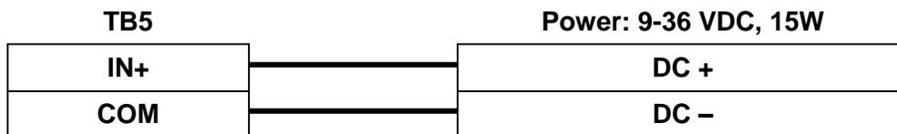
**Figure 10 - DC Power Supply Connection**
