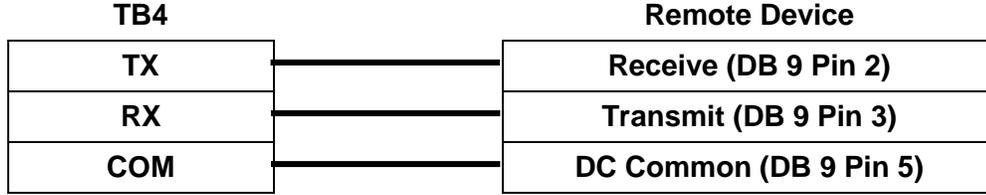
Figure 27 - RS-232 Serial Interface
