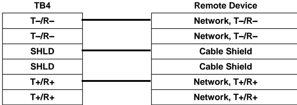
Figure 28 - RS-485 Serial Interface
