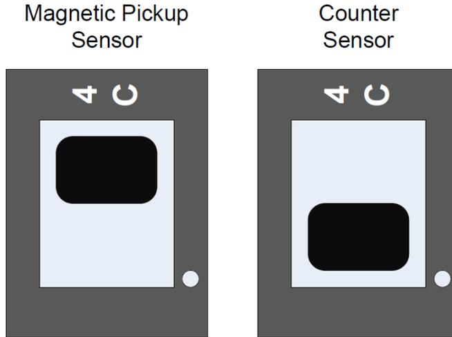
**Figure 19 - Count Sensor Interface DIP Switch Positions**
