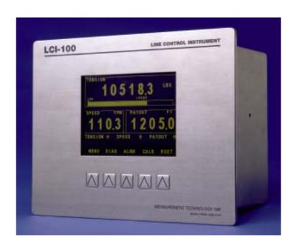
The LCI-100 is a full-featured instrument that offers exceptional performance and readability in demanding environments from -40°C to +75°C. Its multi-channel capabilities allow for future expansion, and its bright 320x240 electroluminescent display permits wide-angle readability of tension, payout, and line speed status regardless of the lighting conditions.
